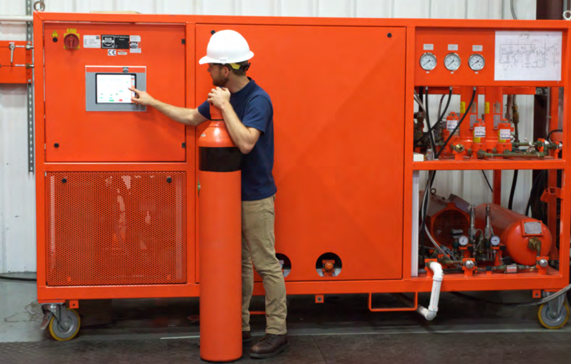
Figure 1: SF 6 gas separator, which uses a cryogenic process to recondition contaminated SF 6 gas to >99.99% purity
