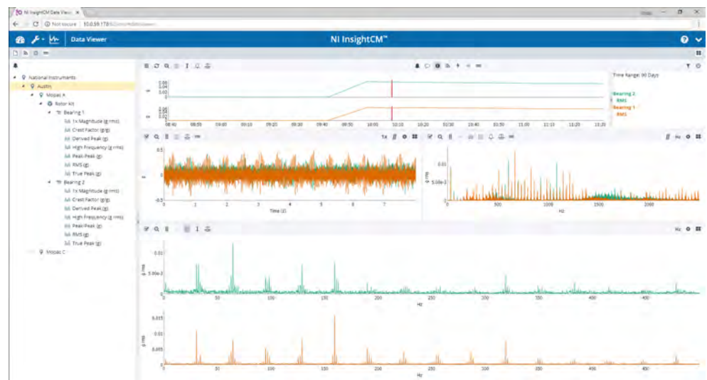
Figure 1: Vibration measurement layout showing RMS trend line, waveform, spectrum and envelope analysis
