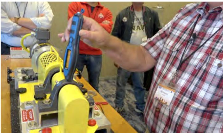
Figure 2: Vibration readings taken "as found," before work and "as left," once work is completed
