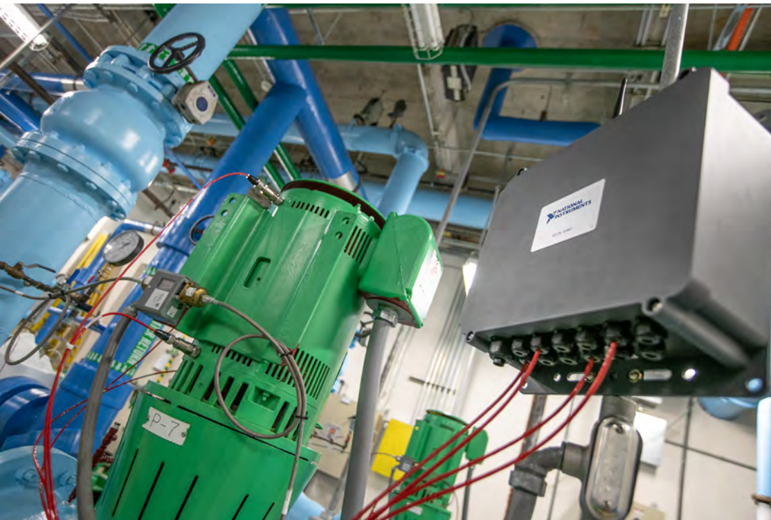
Figure 3: Wireless instrumentation shown connected to standard, piezoelectric accelerometers reduces the cost of high quality waveform data
